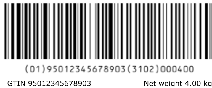
Figure 7.8.6.1-2. Data encoded in one concatenated GS1-128 symbol
