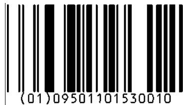
Figure 5.5.2.1.1-1. GS1 DataBar Omnidirectional barcode
