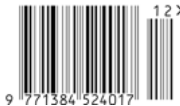
Figure 5.2.2.5.1-2. EAN-13 barcode with two-digit add-on symbol
