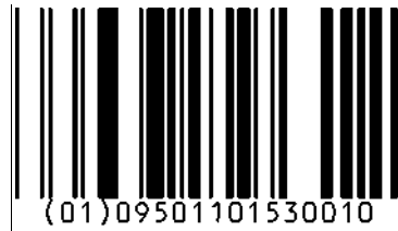
Figure 5.1-4. GS1 DataBar Omnidirectional barcode
