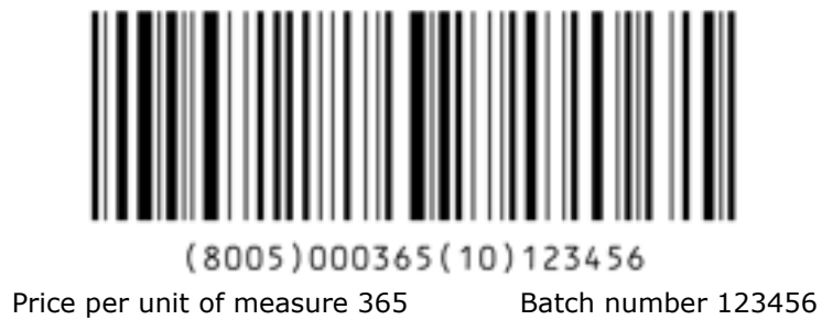
Figure 7.8.6.2-2. Data encoded in one concatenated GS1-128 symbol
