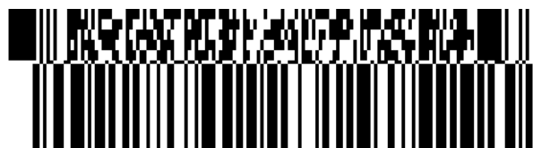
Figure 5.11.2-2. GS1-128 Composite symbol with CC-C
