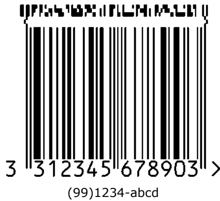
Figure 5.11.8-2. UPC-A symbol with a four-column CC-B component
