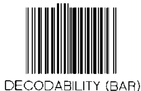
Figure 5.12.5.12-3. Calibration symbol with engineered low decodability grade
