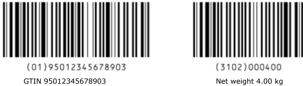
Figure 7.8.6.1-2. Data encoded in one concatenated GS1-128 symbol
