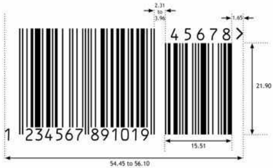
Figure 5.2.6.6-6. EAN-13 barcode with five-digit add-on symbol
