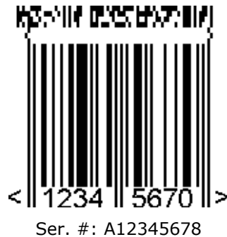
Figure 5.11.8-4. UPC-E symbol with a two-column CC-A component
