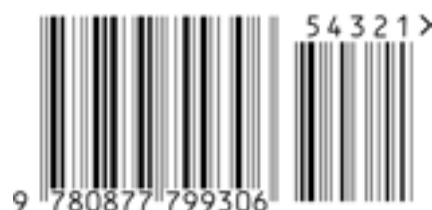
Figure 5.2.2.5.2-2. EAN-13 barcode with five-digit add-on symbol
