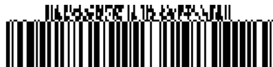
Figure 5.11.8-9. GS1-128 symbol with a four-column CC-A
