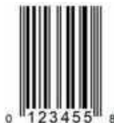
Figure 5.2.2.4-1. UPC-E barcode (encoding 012345000058 by zero-suppression)
