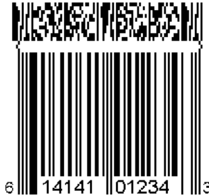
Figure 5.11.8-3. EAN-8 symbol with a three-column CC-A component
