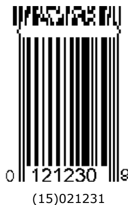
Figure 5.11.8-4. UPC-E symbol with a two-column CC-A component
