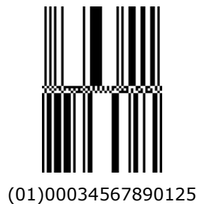
Figure 5.5.2.1.4-1. GS1 DataBar Stacked Omnidirectional barcode
