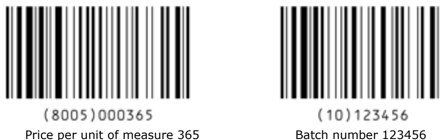
Figure 7.8.6.2-1. Data encoded in two GS1-128 symbols
