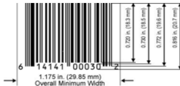
Figure 5.12.6.3-1. EAN/UPC symbol shown with minimum height and overall width dimensions for magnifications of 75 percent to 80 percent
