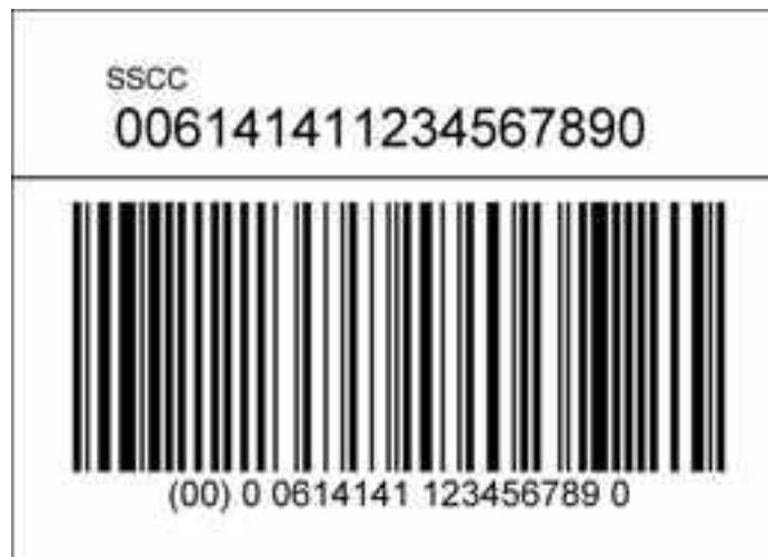
Figure 6.6.5-1. The basic label: an SSCC
